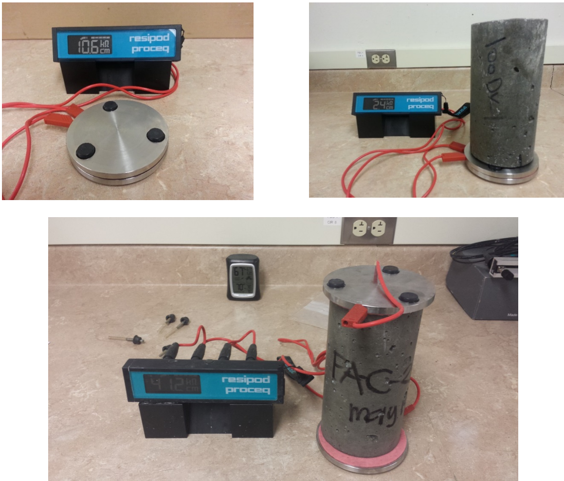
Figure 15. Measuring bulk electrical resistivity. Top foam (top left), lower foam (top right), and specimen resistivity (bottom).
