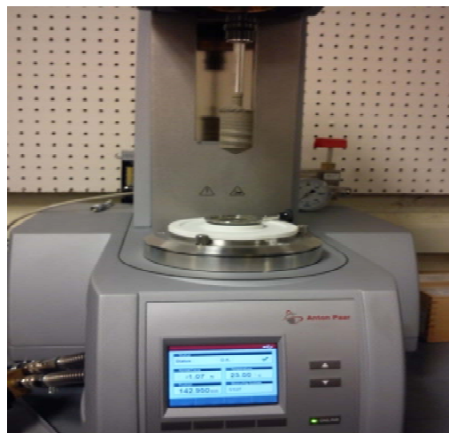
Figure 6. Anton Paar MCR 302 Rheometer used to determine the rheological properties of cement pastes.
