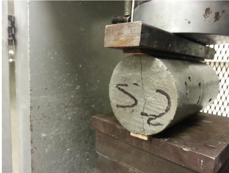
Figure 10. Splitting tensile strength setup.
