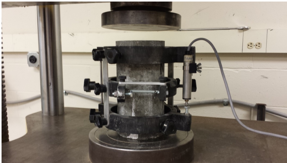
Figure 9. Test set-up of modulus of elasticity test.
